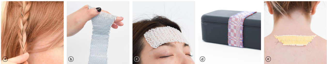
Figure 1: We present EcoThreads, a sustainable e-textile prototyping approach for fabricating biodegradable functional threads. We demonstrated five sample applications: (a) Braided capacitive touch sensing hair accessory. (b) Woven pH-sensing underwear. (c) Woven heat sensing bento box band. (d) Knitted cooling gel for fever. (e) Woven sweat rate sensing patch.
